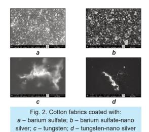
As shown in figure 2, barium sulphate applied cotton fabric (figure 2, *a*) and barium sulfate-nano silver applied cotton fabric (figure 2, *b*) 3000 times, tungsten applied cotton fabric (figure 2, *c*) 5000 times, tungsten-nano silver applied cotton fabric (figure 2, *d*) 1000 SEM image was taken enlarged.
